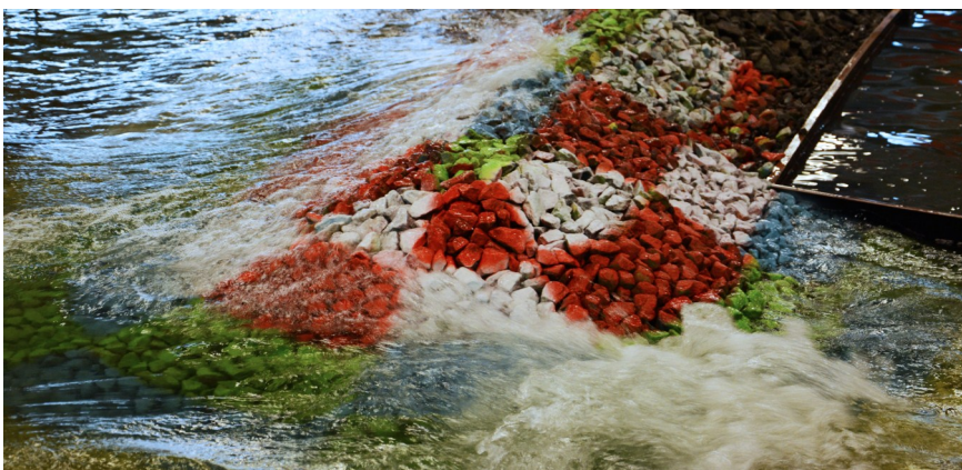
Three-dimensional physical modelling of breakwater head in severe storm conditions. © DHI
