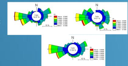
Figure 7- Modeling resulted current roses for 3 points shown in figure 5
