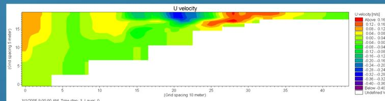
Figure 3- 2-D plot of U-velocity component for a specific time step along the eastern boundary taken from the NCOM model as the boundary condition
