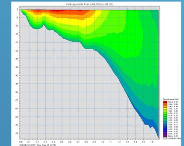
Figure 6- Modeled current speed depth profile along the transect shown in Figure 5
