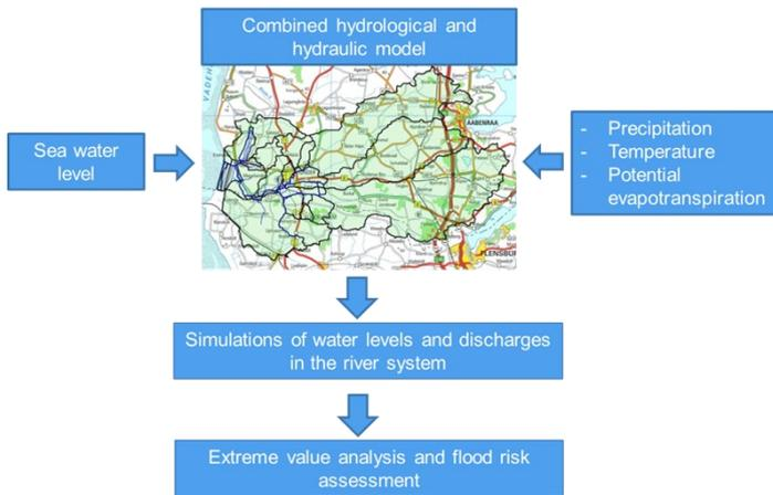
Illustration of the modelling approach. The hydrological and hydraulic model is forced with climate and sea water level time series representing current conditions and future 2050 and 2100 conditions
